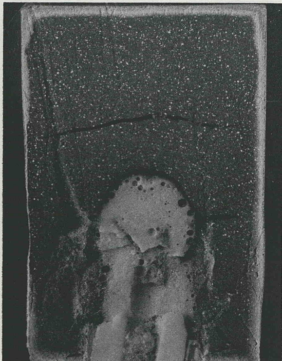
Fig. 6. Cross section of 50% \text{Al}_2\text{O}_3 and 50% \text{TiO}_2 thermite pellet.
